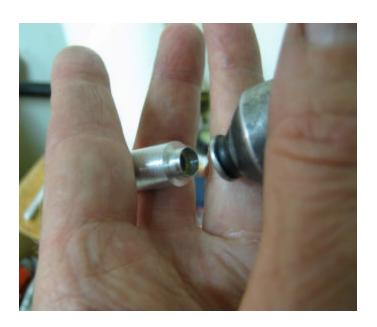
Fig3: Turn down the outside diameter for a snug fit into the end of the muffler. It's a good idea to measure an assortment of mufflers in advance. Although the rules state a maximum outlet diameter of 8 mm, many of the mufflers may be undersize. It's much easer to turn down the O.D. of the insert at this stage than once the part is finished.
