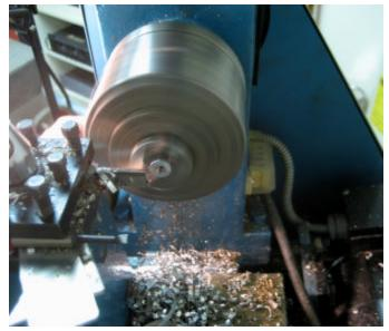
Fig4: Turn the part around and carefully re-chuck into the lathe. The wall thickness will be quite thin now (just the difference between the approximately 8 mm O.D. and the 9/32" internal hole). Cut off the part, leaving a 1/16"-3/32" flange with the smaller (6 mm) I.D. hole.
