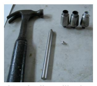
Fig8: To install, you will need a long punch (narrow enough to fit inside a muffler), and a hammer.
