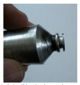
Fig9: Slip the insert into the end of the muffler.
