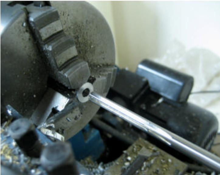
**Fig5: Ream the hole to exactly 6 mm**
